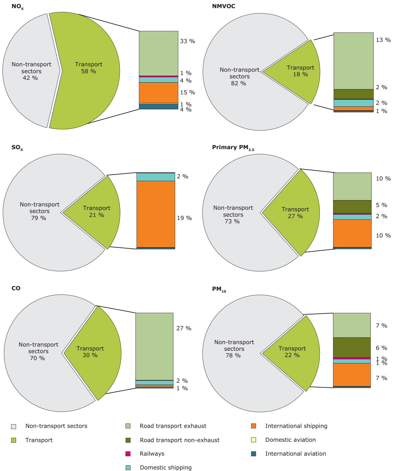
Figure 4.1 The contribution of the transport sector to total emissions of the main air pollutants in 2010 (EEA-32)
