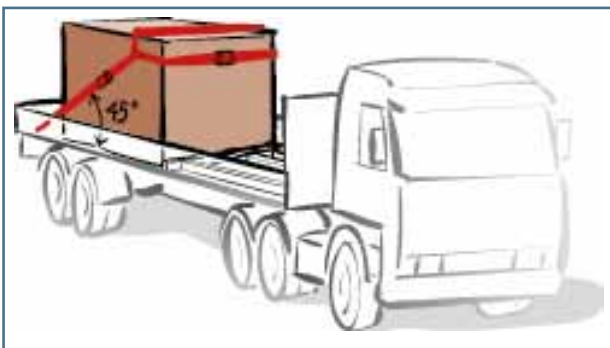
Fig. 26. Example a spring lashing preventing forward movement
