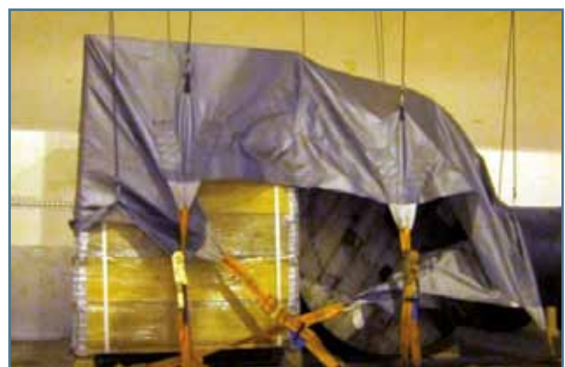
Fig. 42. Restraint system with integrated lashings
