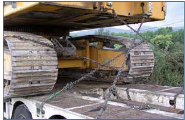
Fig. 39. Excavator diagonally lashed with chains
