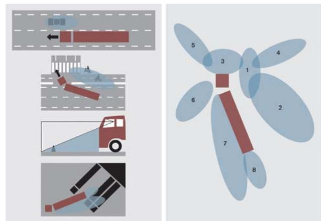
Figure 4. Truck seen from above. The numbered fields, 1–8, show areas that can be difficult for the driver to see.
