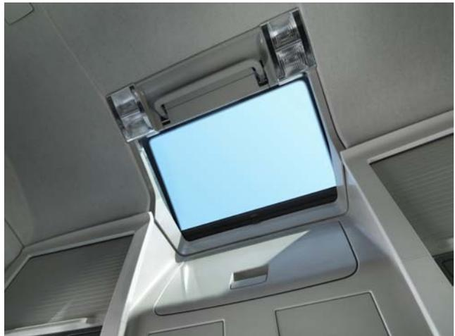
Figure 7: The roof hatch in the new FH functions as escape path in case of a vehicle roll over accident.
