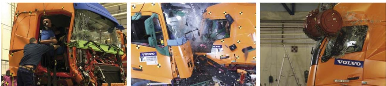
Figure 2: An illustration showing the knowledge gained from crash tests (crash facility testing, full scale test of new FH, pendulum testing) and a picture showing the investigation of an accident in the field.
