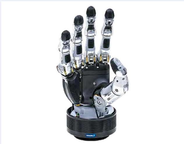
Figure 20: Servo-electric 5-finger gripping hand; Source: Schunk
