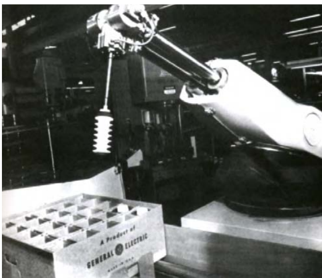
Figure 4: The Unimate on the General Motor's assembly line in 1961; Source: Computer History Museum
