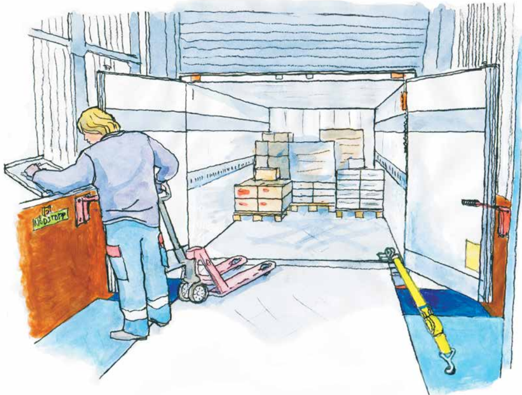
Loading house with step bridge, allowing an unbroken cold chain.
